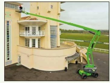
The HR28 Hybrid 4x4 also incorporates Niftylift's multi award winning SiOPS® safety system. SiOPS® eliminates sustained involuntary operation by instantly stopping machine movement if the operator is pushed onto the control console, allowing them to safely recover their situation.
