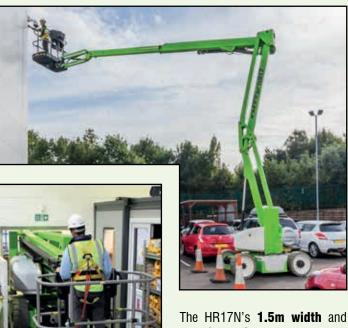
The HR17N's **1.5m width** and **sub 2m height** enables travel through restricted spaces. Optional non-marking tyres mean that it can work both inside and out making it ideal for industrial or maintenance work.
